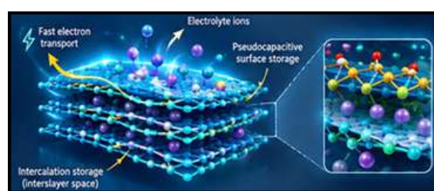
Fig. 3: Energy Storage Mechanisms in 2D Layers
